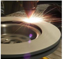
industry is currently seeking for better and cheaper approaches to controlling these problems. Coating technology remains a method by which the wear resistance of components can be improved. In this study, different carbides materials had already been coated on the friction surfaces of several GCI brake discs via extreme high-speed laser (EHLA) material deposition. The tribological and wear performances of coated discs are yet to be analyzed and evaluated, which are the focus of this study.
